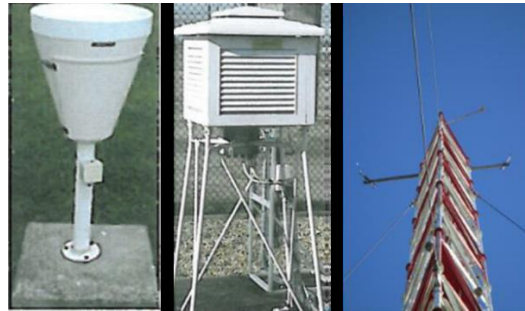
Examples of rainfall, temperature and wind measurement equipment ©EDF
